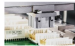
Force-feedback final Press/seating
